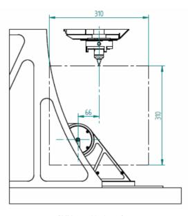
μCMM – positioning volume with μCMMReal3D, side view, Y axis in middle position
