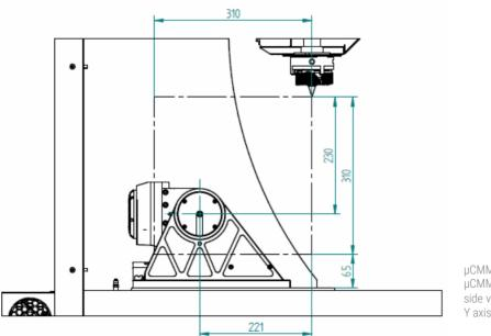
μCMM – positioning volume with μCMMReal3D, side view, Y axis in rearmost position
