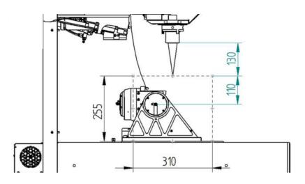
μCMM – positioning volume with μCMMReal3D and μCMMObjective 1500 WD130, side view, Y axis in middle position
