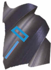
ToolRoughness Roughness measurement on rake and clearance surface
