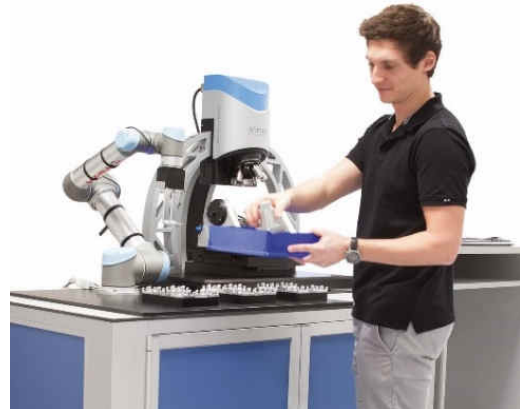
High-resolution optical 3D measurement technology in combination with a collaborative robot arm enables automated placing, measuring and OK/NOT OK sorting in production.
