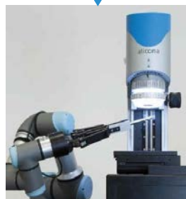
Automated placement and measurement with turbine blades
