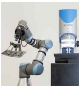
Automated placement and measurement with turbine blades
