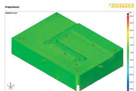
3D measurement of a die, performed with Alicona's high-resolution optical measuring system InfiniteFocus.
