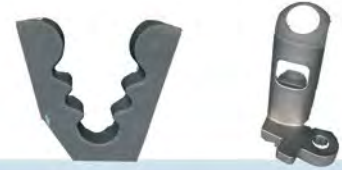
3D visualization of a turbine disc fir-tree root. Deviations are automatically measured so that out-of-tolerance features are quickly assessed. 3D visualization of an injector combustion chamber. The optical measurement system by Alicona is used to verify geometry, positioning and functional dimensioning.
