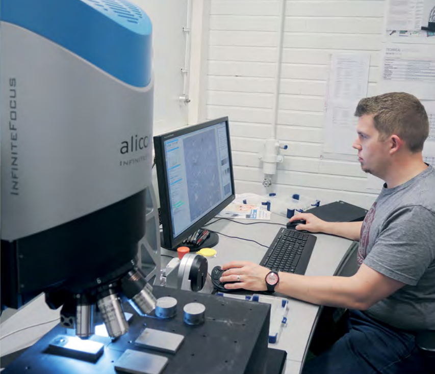
Niko Ojala , researcher at the Laboratory of Materials Science at TUT; using MultiMeasurement: With InfiniteFocus G5 Ojala defines the measuring routine with which several specimens are automatically measured one after another.
