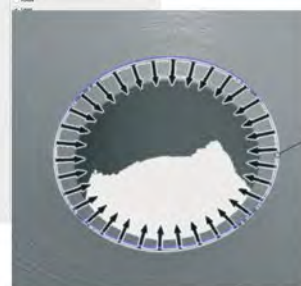
Sphere with a defined diameter (1.5 mm) is projected onto the data set, including displayed contact surface.
