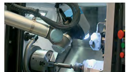
... and first measures predefined cutting edge parameters of the insert.
