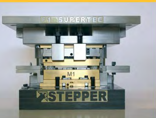
Stepper stamping tool to manufacture contact parts for the automotive industry. 16,100 contact parts per minute can be produced.
