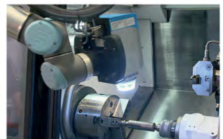
The sensor then moves on to the workpiece and measures its roughness to verify surface quality. Then the robot arm returns into its original position. All measurements are carried out without unclamping components.
