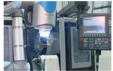
... and a further signal sets the Cobot in motion. The robot arm with 3D measuring sensor is automatically manipulated into the lathe...
