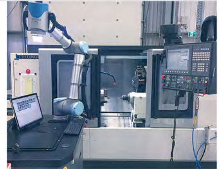
A central control system starts the testing process. At a defined point the lathe stops, the door opens...
