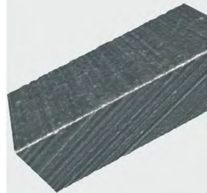
3D measurement of a milling cutter produced by laser processing.
