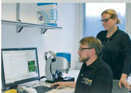
Measurement of special milling tools with Alicona - Corinna Ruess and Manuel Herrmann
