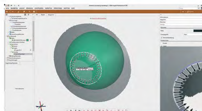
Sphere with a defined diameter (1.5 mm) is projected onto the data set, including displayed contact surface.
